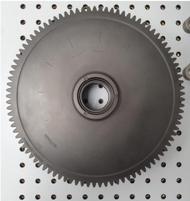
The burns were revealed by nital etching prior to NV measurements.
